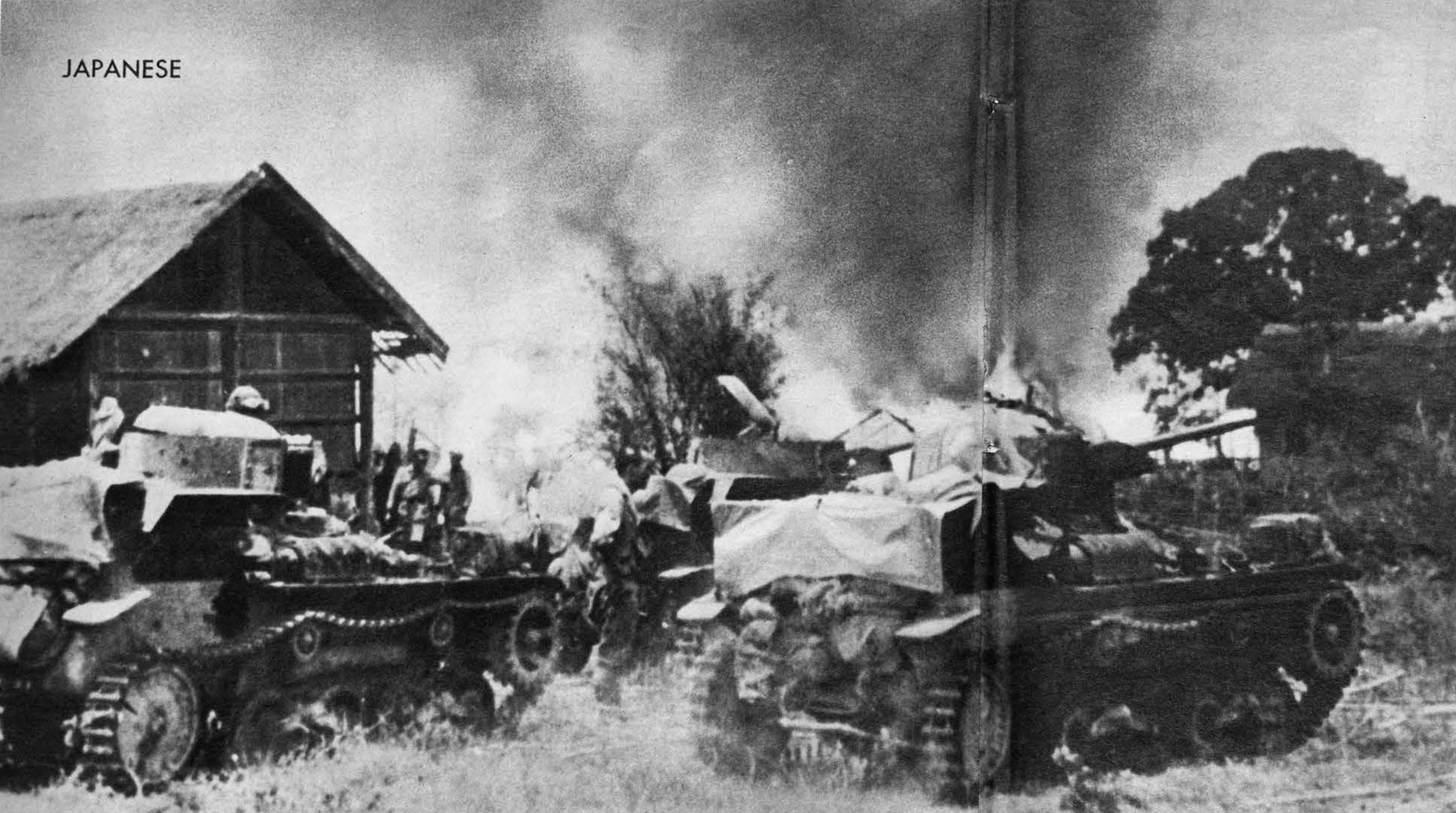
The 2597 is first of series to mount 37-mm. cannon in turret. Its large rear idler provides greater ground traction. The later models may have heavier armor plate, wider track, and an intercommunication system.
